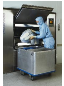
Hepa filtered Dryer
