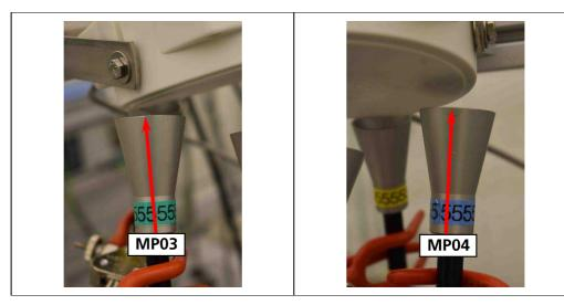
Figure 5 Measuring points MP01 to MP04 selected to measure airborne particle emissions from TP01
